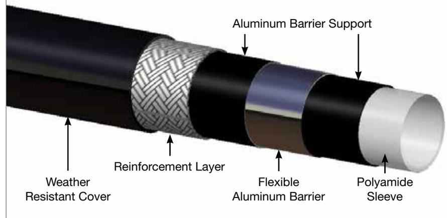
**ZoomLine** has been designed to eliminate refrigerant leakage while maintaining flexibility not available with copper tubing. The 6 layer hose is designed to withstand environmental, temperature and pressure extremes while providing excellent installation flexibility and long life.
